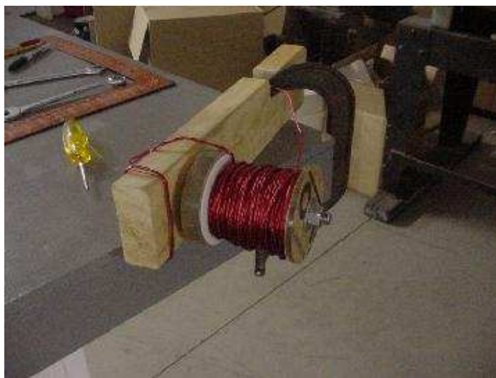
Winding the coils on the coil winding jig
