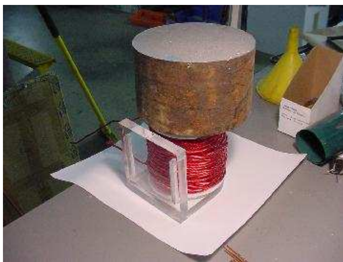
Coil being glued to mounting base under pressure
