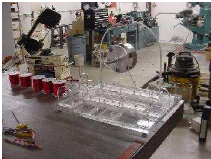
Coils wound and mounting bases finished
