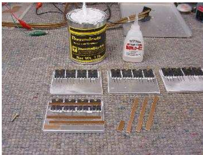
Mounting the switching circuits.
