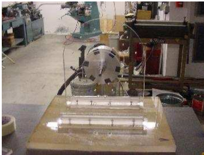
Front view of rotor with magnets
